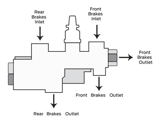
While this Proportioning Valve will work for all applications, for vehicles with front disc brakes and rear drum brakes, Proportioning Valve (P/N: C5ZZ-2B091-R) is recommended.
